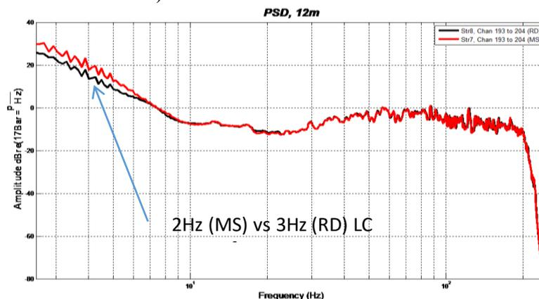
**Figure 2** Noise amplitude spectral display comparing a 3 Hz low-cut hydrophone-only solid cable section (black) to the 2 Hz low-cut hydrophone channels of multi-sensor solid cable section (red). Data recorded at the same time on two adjacent streamers, with the same offset.
