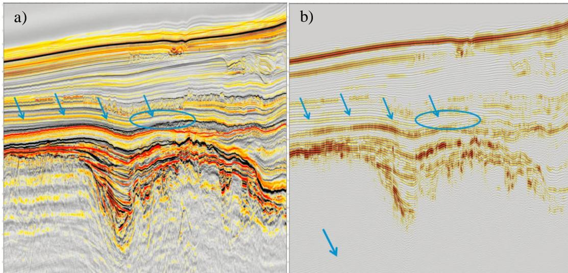
**Figure 3** Data example after migration using hydrophone-only deghosting: a) Full bandwidth, b) Band-pass filter around hydrophone notch (62.5 Hz)
