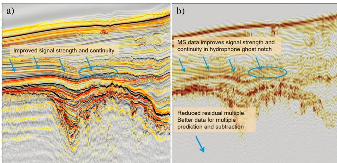
**Figure 4** Data example after migration using joint deghosting: a) Full bandwidth, b) Band-pass filter around hydrophone notch (62.5 Hz)
