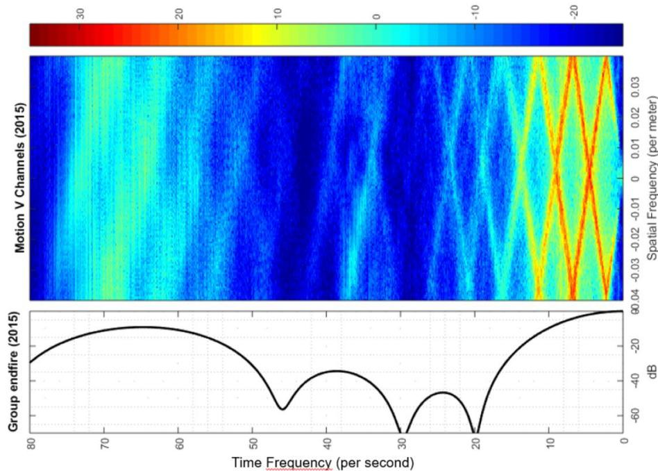
**Figure 1** F-K plot of motion data recorded during tow noise test that shows the effective attenuation of the higher frequencies of the transverse noise by the sensor array.
