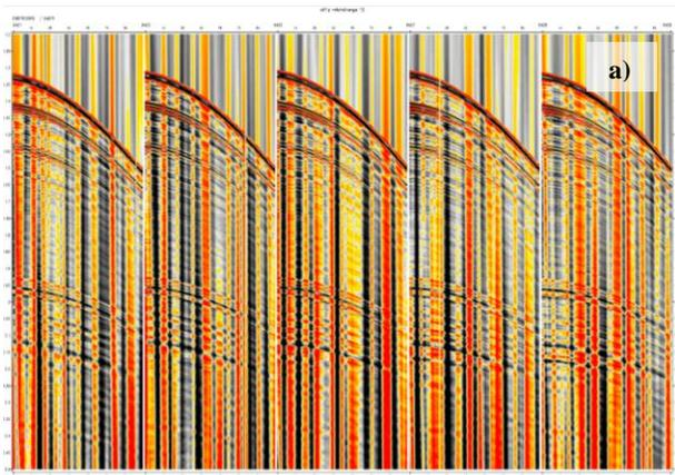
For the accelerometer data it is obvious that more noise attenuation is required. Figure 4 a) and b) show the same data as Figure 3 but after a more elaborated noise attenuation than a simple lowcut filter.
