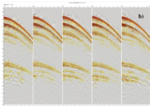
Figure 4: The same field records as shown in Figure 3 with a more elaborated noise attenuation method. a) Hydrophones, b) Accelerometers (vertical component)
