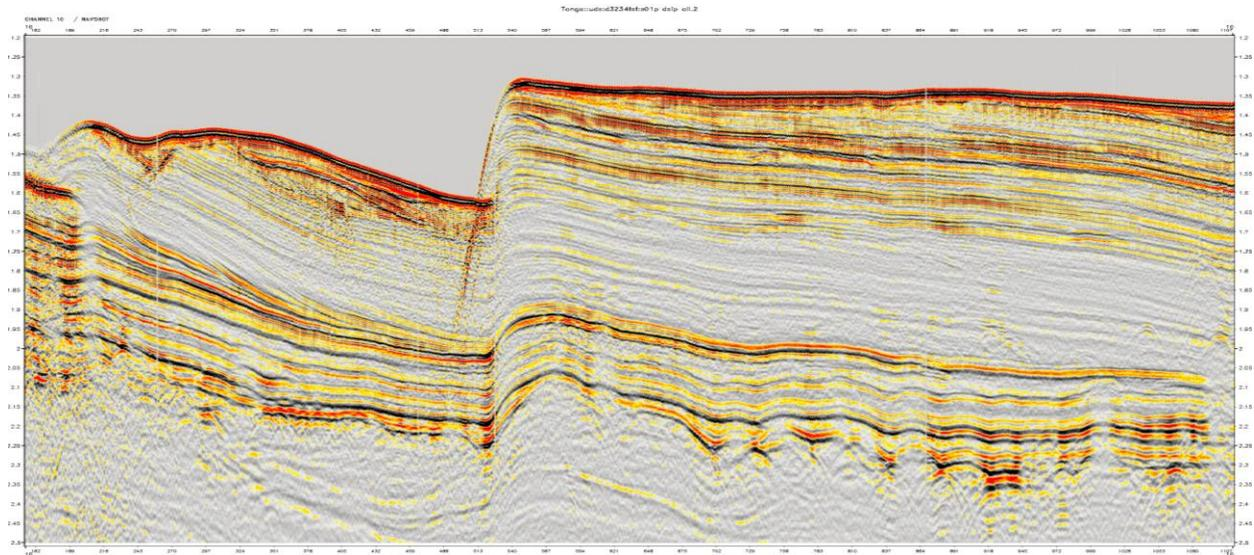
Figure 5: A single fold, short offset gather of the hydrophone data after noise attenuation along a portion of the test line.
