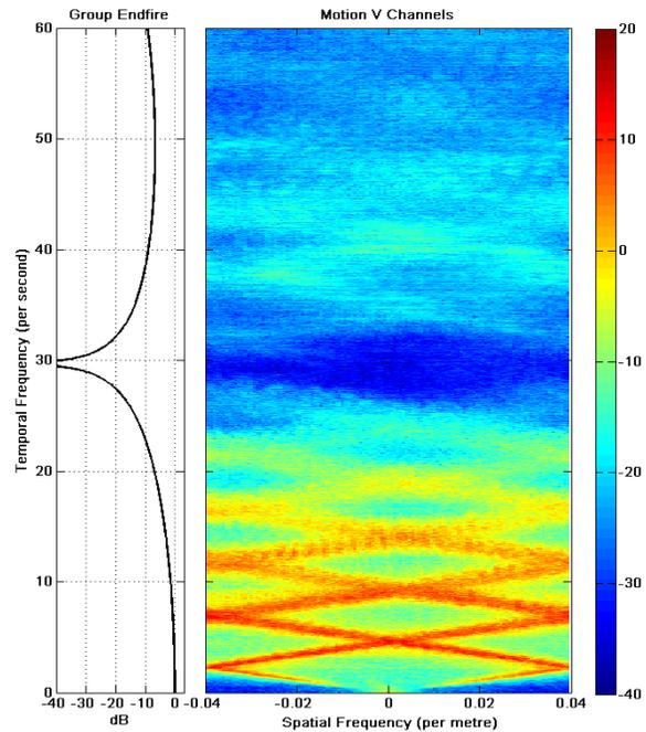
Figure 1: F-K plot of motion data recorded during tow noise test that shows the effective attenuation of the higher frequencies of the transverse noise by the sensor array.
