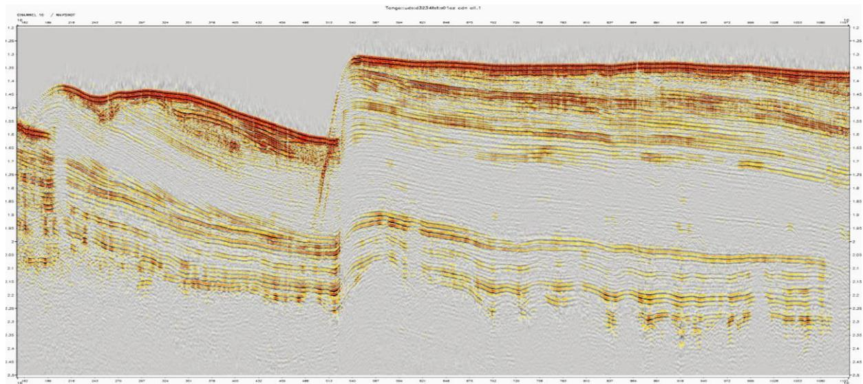
Figure 6: The same portion of the test line as shown in Figure 5 but showing the vertical accelerometer data after noise attenuation.
