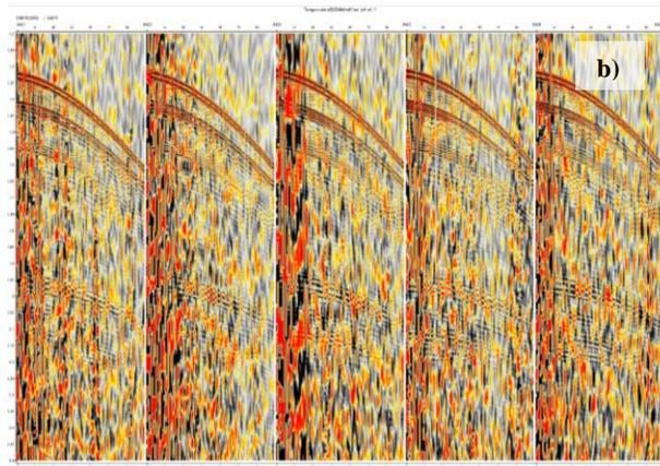
Figure 3: Displays of portions of five raw shot records with no noise attenuation. a)Hydrophones, b)Accelerometers (vertical component) accelerometer data showing a much higher frequency content.
