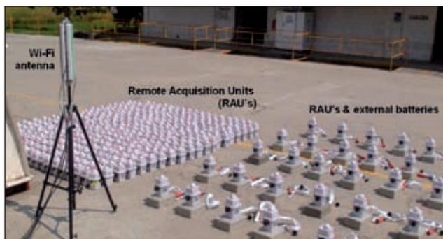
Figure 1 Cableless system made of RAUs communicating with a Wi-Fi antenna for set-up, quality controls, and data harvesting.
