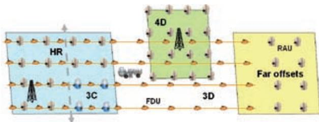
**Figure 4** Multi-spread configuration: a cable system (FDU) is completed by RAUs to locally increase spatial sampling (HR), to change the type of sensor (3C), or to record far offsets. Continuous monitoring (4D) of production may also be performed.
