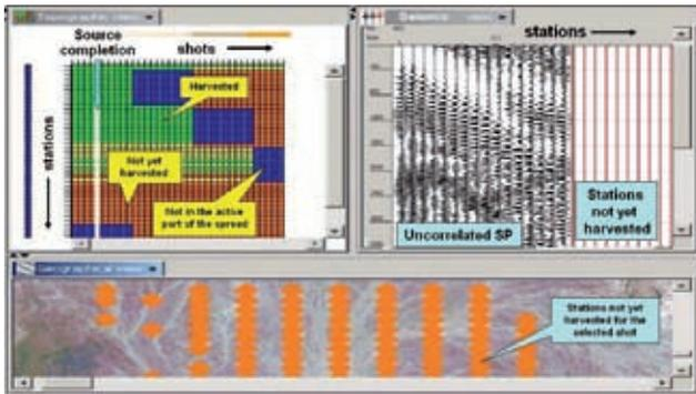
**Figure 3** Data off loader (DOL) interface for a cableless system. The table view (each case corresponding to a seismic trace) is completed by the display of seismic data selected in the table and by a GIS interface with the location and status of the RAUs.
