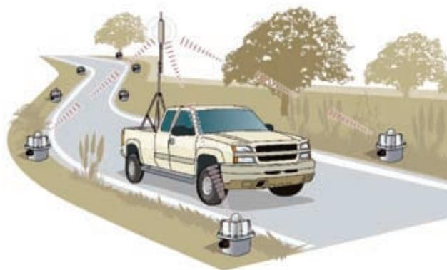
Figure 2 Mobile harvesting (patent pending) using a pick-up equipped with a Wi-Fi antenna.
