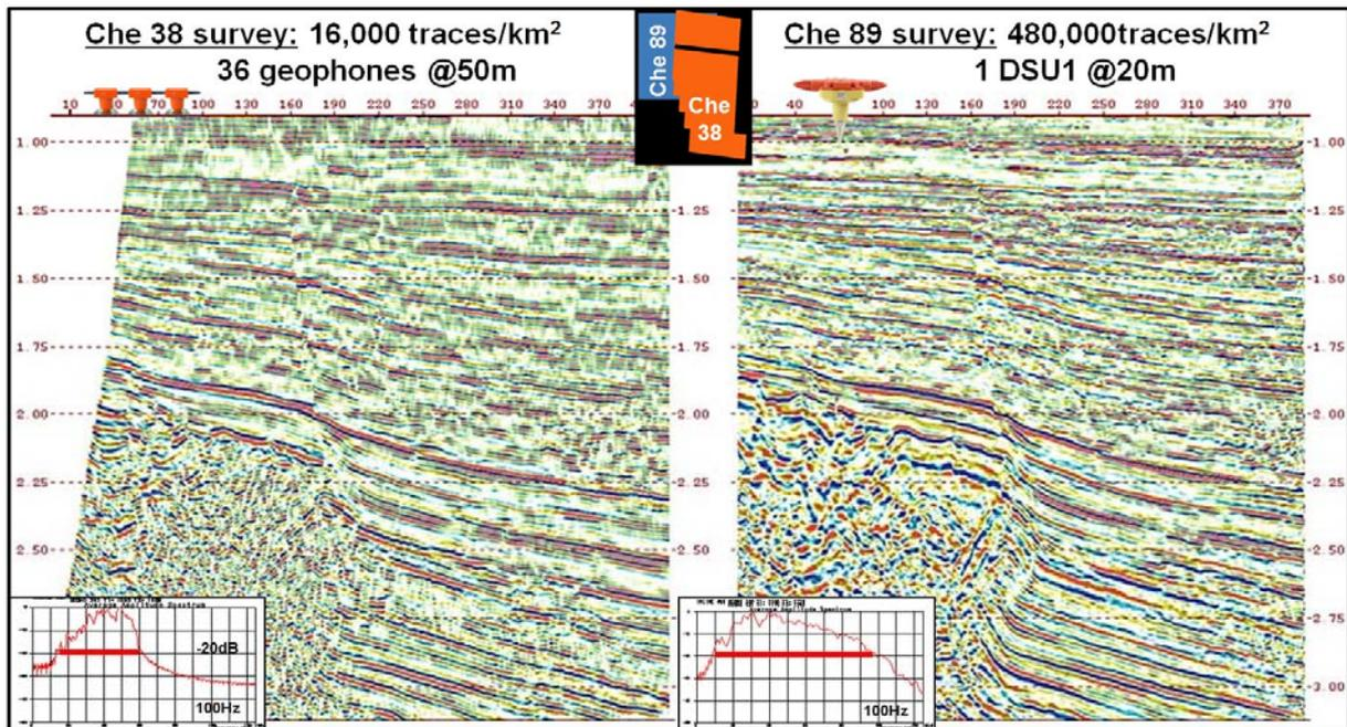
Figure 1: Benefits of single sensor high-density 3D acquisition to improve vertical resolution and seismic imaging.
