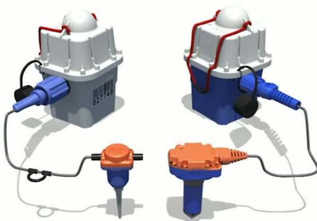
**Figure 1:** UNITE cableless system is proposed in various configurations: to the left the RAU is connected to an analog geophone, to the right the RAU-D powers a 3C digital accelerometers (DSU3SA).
