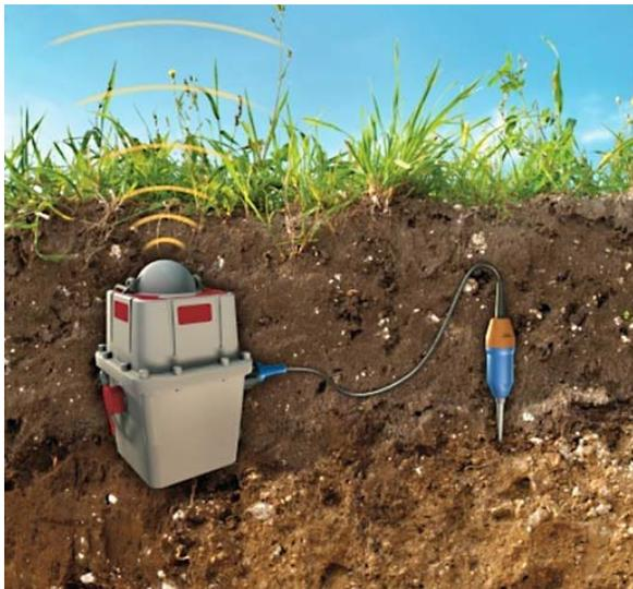
to reach two weeks autonomy (10h/day) without external battery. This option combined with a single geophone offers a configuration that may be more easily buried with the top of the RAU 10cm down the ground surface while all GPS and WiFi capabilities are kept (Figure 2). In the snow or in dry sand the burying depth may be even higher.
