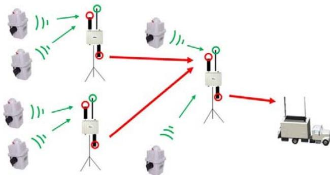
**Figure 6:** for full real-time data transmission, a Mesh network is used. It is composed of nodes, each one collecting RAU data at 2.4 GHz (green) that are propagated between antennas at 5.8 GHz (red).
