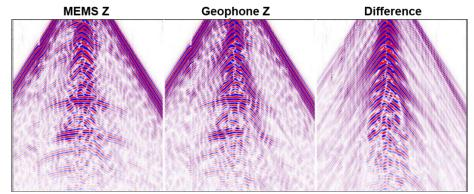
Figure 1: Example of CRG in m/s, 16-31 Hz bandpass filter, time window 0.5-2.2 s.
