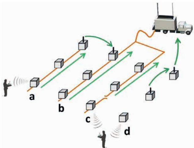
**Figure 6** Cross-technology recorders mix the possibilities described in figures 2 to 5 within the same spread: (a) autonomous line with no physical connection to the central unit, (b) cabled line connected to the central unit, (c) cables line with line cut and (d) line of wireless channels.
