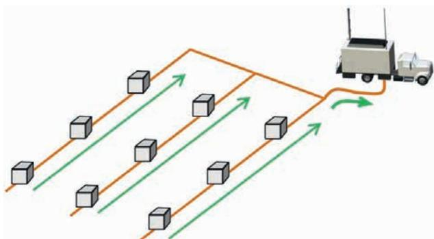
**Figure 2** Cable recorders have a centralized architecture: seismic data and QC are available in real-time.
