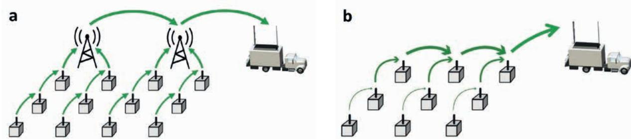
**Figure 3** Real-time and remote QC wireless recorders can be based on two architectures: (a) relay antenna backbone and (b) multi hops.
