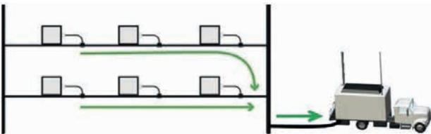
**Figure 5** Blind wireless recorders: QC available only through physical connection (usually on racks) after modules are retrieved from the field.
