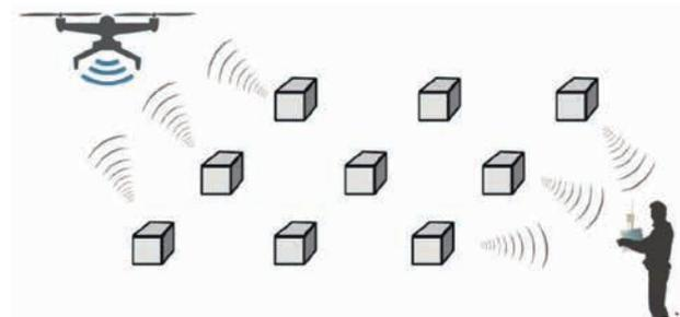
**Figure 4** QC capable wireless recorders: seismic data and QC can be harvested on the field.
