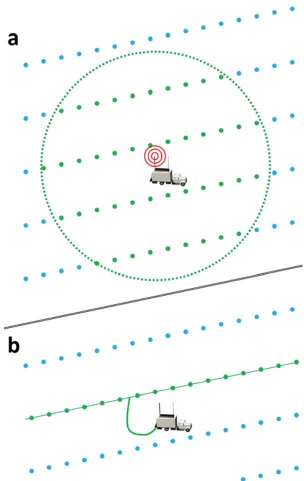
**Figure 9** (a) seismic data and operation QC collection around recorder. Extra antennas (not represented) can be installed. (b) a wireless spread complemented by a cabled line. With these two solutions, both data and operation QC are available in real-time. Channels harvested are displayed in green.
