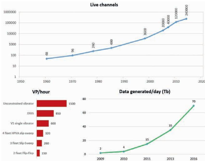
**Figure 1** Evolution of land acquisition parameters. Increasing channel count and productivity generates more data: its QC has to be adapted.
