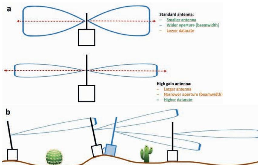
**Figure 10** (a) comparative radiated power of a standard large aperture antenna (up) and high-gain narrow aperture antenna (down). Only major lobe is shown. (b) field preparation with narrow aperture antennas: antennas have to be aligned, and repeaters (blue) used in case of uneven topography.
