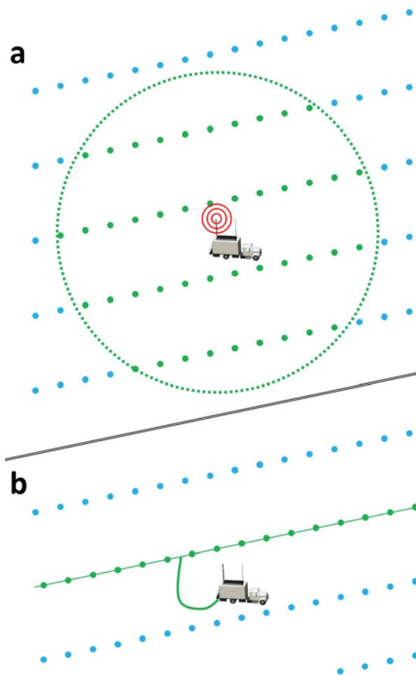
**Figure 9** (a) seismic data and operation QC collection around recorder. Extra antennas (not represented) can be installed. (b) a wireless spread complemented by a cabled line. With these two solutions, both data and operation QC are available in real-time. Channels harvested are displayed in green.
