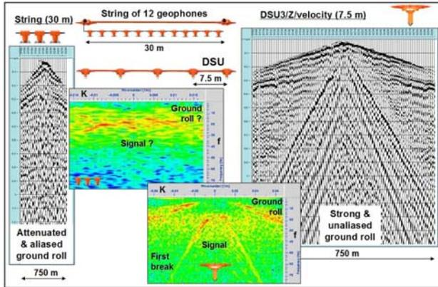
Figure 1: Shot points over the same offset range from strings of geophones (left) and digital sensors (right). FK diagram shows that the prominent ground roll from single sensor data will be easily removed contrary to the aliased geophone data.
