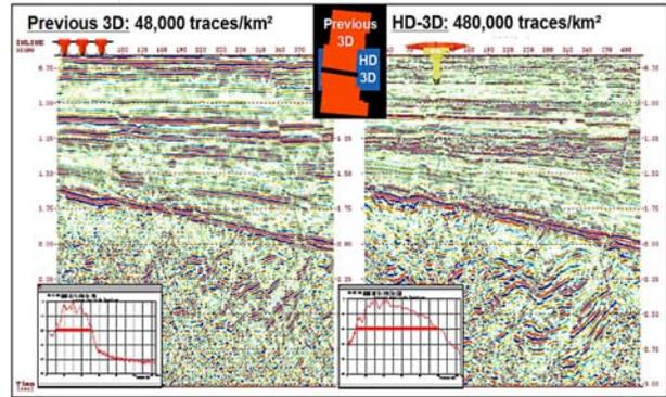
Figure 3: Comparison between two overlapping 3D surveys (Li, J. et al., 2009): one low density recorded by strings of geophones (left section) and a new high density one (HD-3D) recorded from digital sensors (right section). Both vertical resolution and signal-to-noise were improved down 3s twt by HD-3D.
