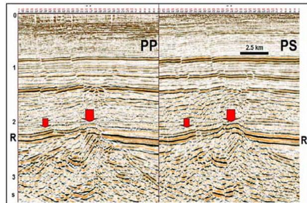
Figure 5: The PS migrated sections scaled to PP time is of sufficient quality to be compared with the PP one. Differences of amplitude at the top reservoir are evidenced on the two highs (Liang, S. et al., 2008).
