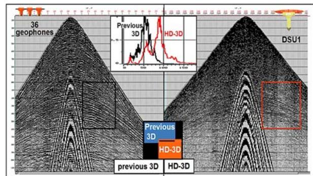
Figure 2: Comparison of SP's between strings of geophones (left) and digital sensors (right), and the corresponding amplitude spectra (Li, J. et al., 2009). The main difference in HF content comes from the comparison of velocity with acceleration data. Ground Roll is attenuated by the array.
