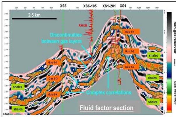
**Figure 6:** Fluid factor section from the PP-PS dual inversion (Liang, S. et al., 2008). The three gas layers as identified at XS-1 & 6 are also evidenced by the positives value of the fluid factor. Thanks to 3C seismic the complex relationships between the two wells are established.
