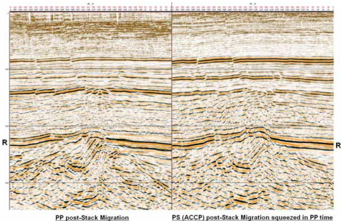
**Figure 4:** Comparison of the PP with the PS post-stack time migration performed from the ACCP stack. PS section was converted in PP time using a gamma zero section. R: reservoir (courtesy of Daqing Geophysical).
