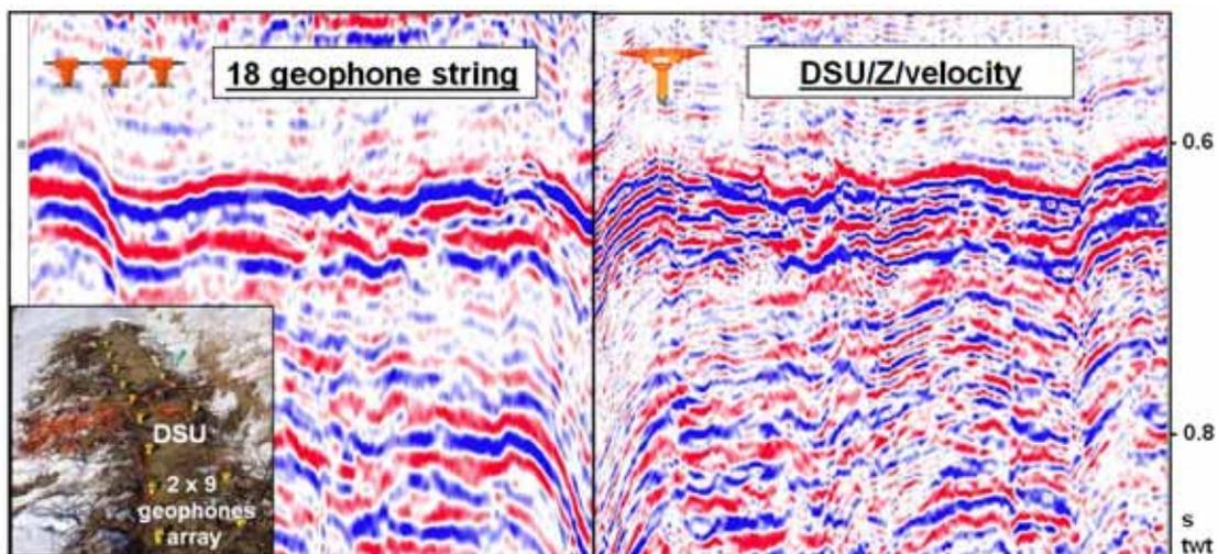
**Figure 3:** Comparison of the vertical resolution on the PP stacks recorded with the same spacing (15 m) between geophone strings (18) and DSU3 (courtesy of Liaohe Geophysical).
