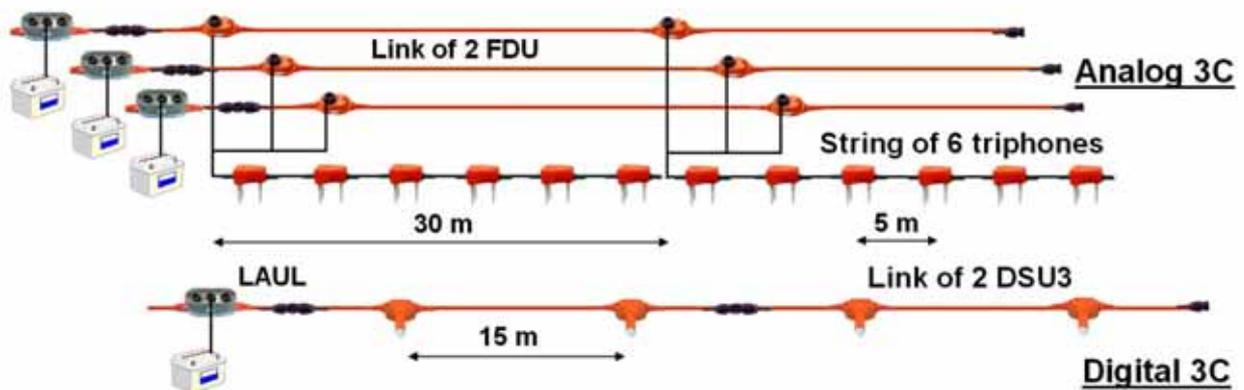
**Figure1:** Comparison of an analogue 3C with a digital 3C line.
