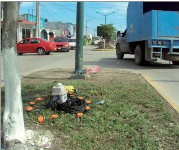
Figure 5 Receiver station planted in median in suburb of the city.
