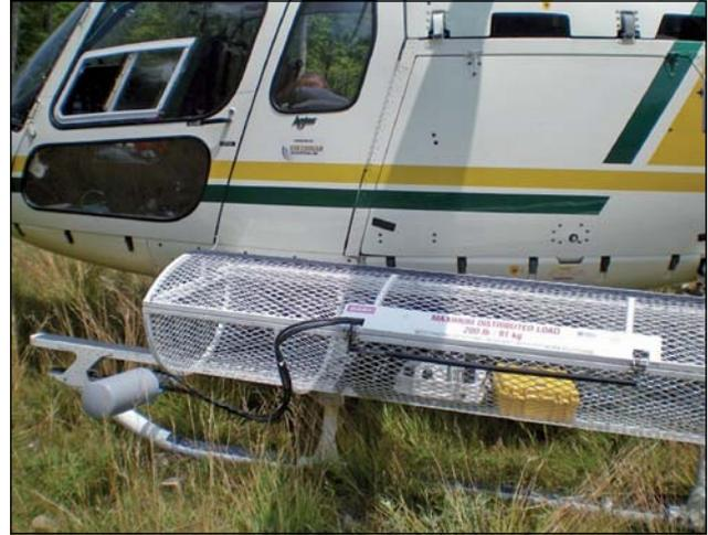
Figure 10 Data harvesting equipment with high gain antenna mounted on basket on helicopter side.
