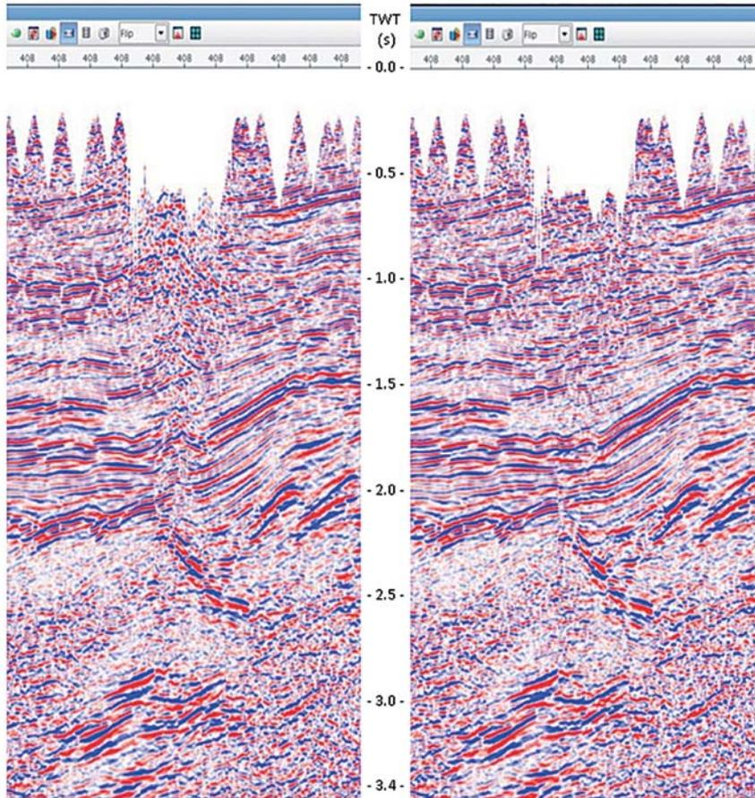
Figure 4 Migrated stacks of CMP line 408, without (left) and with (right) cable-less data.
