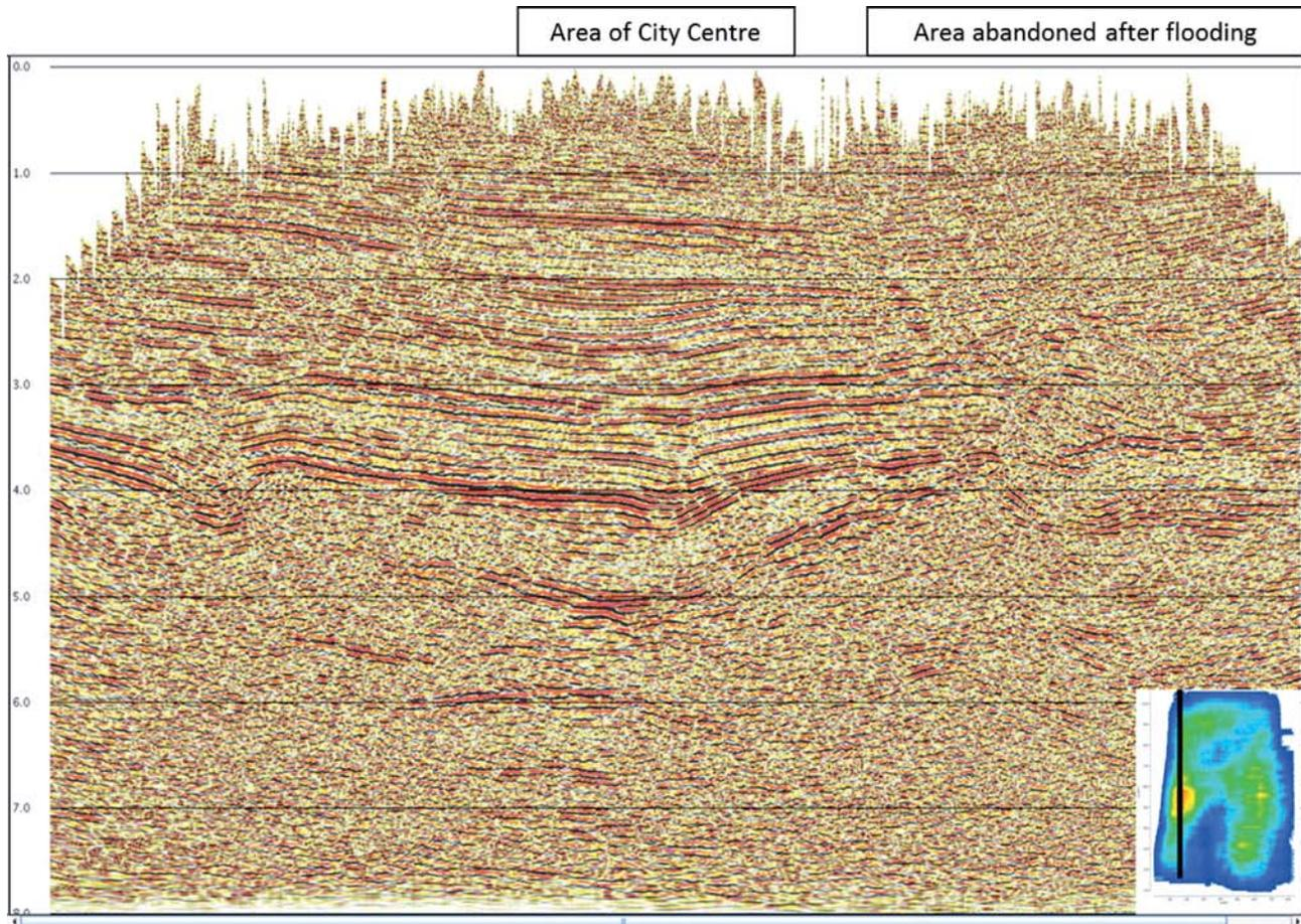
Figure 7 Post-stack QC migration of crossline from the survey. The black line on the inset fold map shows the line location, with the warm colours indicating the higher fold in the centre of the city. The degradation of the data quality on the right corresponds with the lower fold caused by the abandonment of that portion of the survey after the flooding. This is indicated by the blue colours in the South central part of the fold map.
