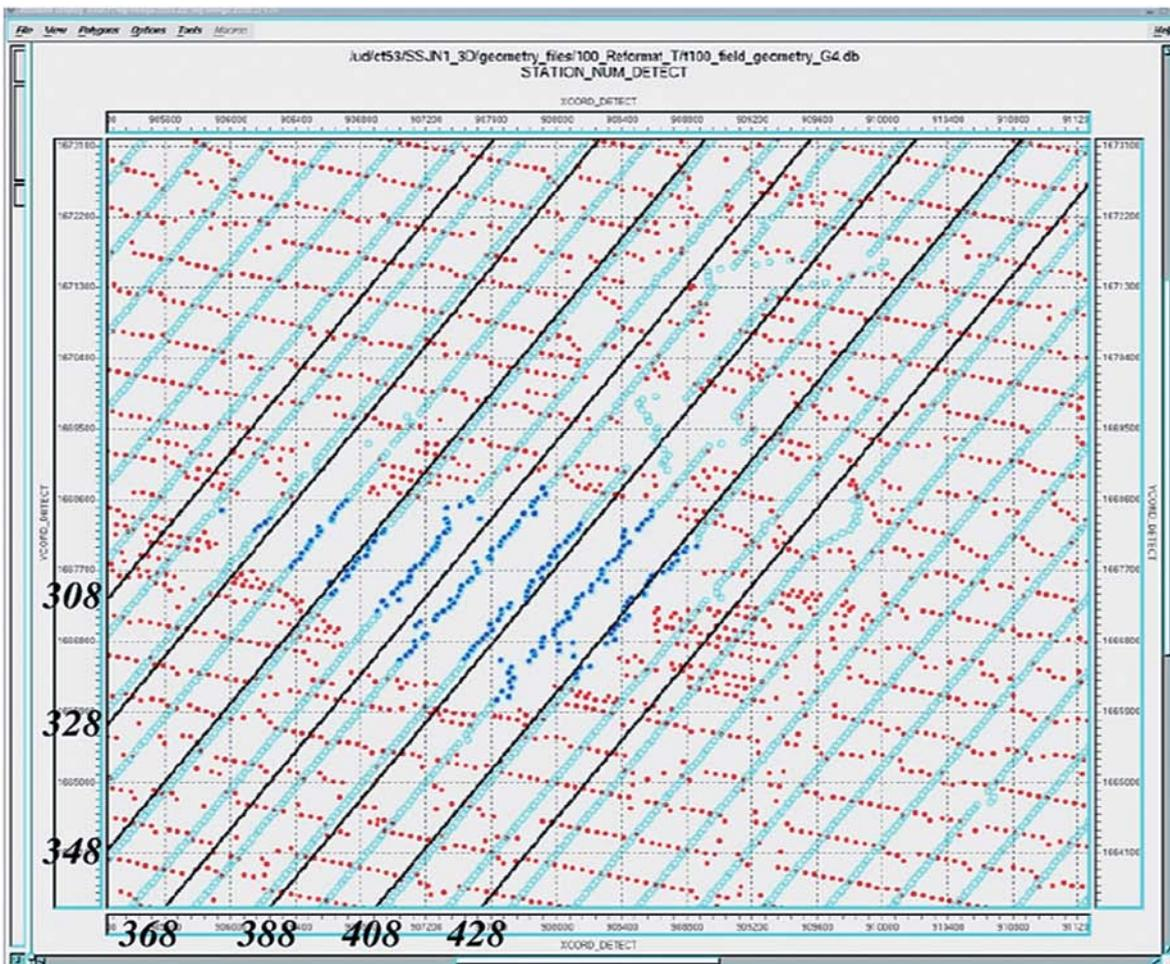
Figure 3 Post plot map of urban area with location and numbering of CMP lines.
