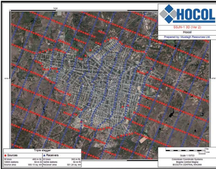
Figure 2 Zoom of pre-plot showing planned geometry through the town.
