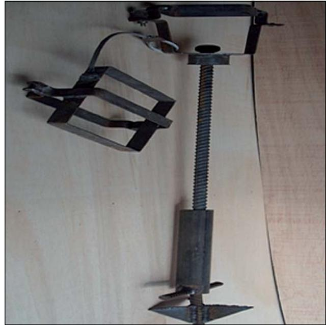
Figure 6 Ground anchor for securing RAUs and batteries.
