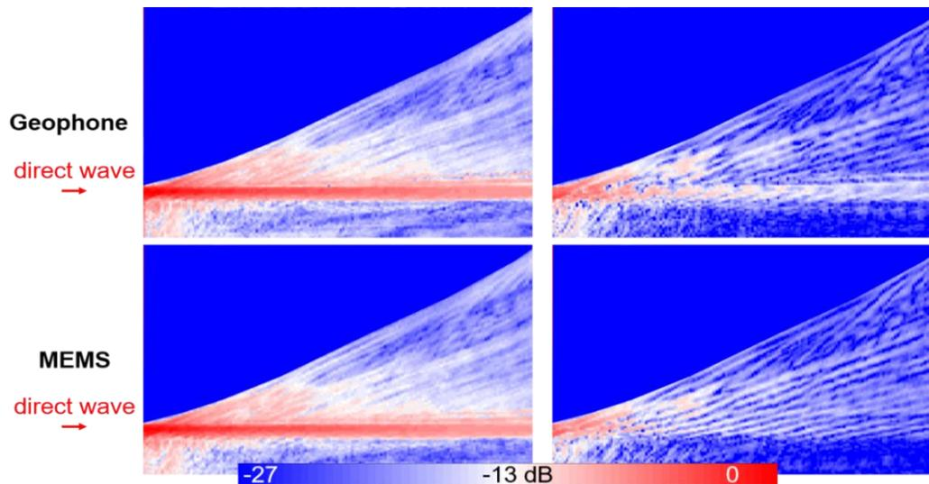
Figure 2: Signal envelopes in dB (m/s) for the geophone data (top) and MEMS data (bottom). (X,Y,Z) envelope (left), and (Z) envelope (right).
