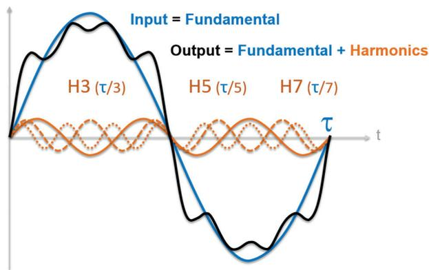
**Figure 1:** an illustration of distorted signal (Output), after the expected “ideal” seismic signal (Input of temporal period  $\tau$ ) has gone through a physical device (source or receiver)
