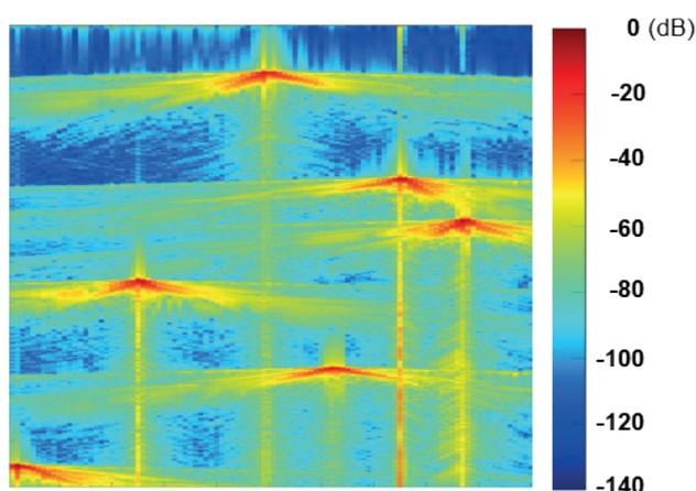
**Figure 3:** Blended seismic operations involve the overlay of seismic signals showing more than 120 dB difference in amplitude.
