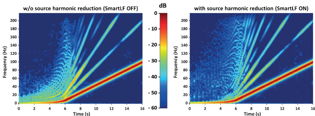
**Figure 2:** Spectrum of the ground force of a shot point, without (left) and with (right) VE464 SmartLF harmonic reduction at the signal emission stage.
