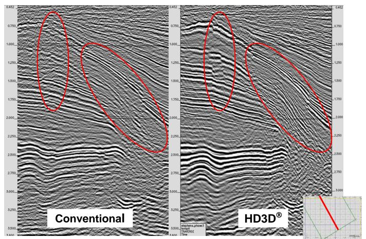
Dip line from conventional dynamite survey. Note: Structural / stratigraphic imaging issues.
