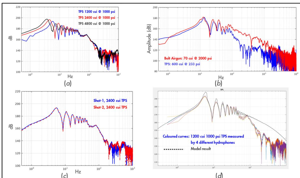
**Figure 3** (a) TPS measurements for different volumes. (b) A comparison between the TPS source and an airgun with the same energy. Note that the TPS is 30 dB weaker at 300 Hz. (c) Repeatability for a 2400 cui TPS source. (d) Modelling results and data from a 1200 cui TPS source.
