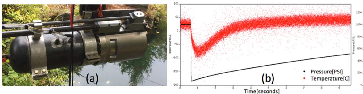
**Figure 2** (a) TPS instrumented with pressure and temperature sensors. (b) Pressure and temperature measured inside the firing chamber of a TPS. The initial pressure of 1000 psi drops to 70 psi. A slow responding temperature sensor indicated that an initial temperature of 20° C drops to -75° C. The firing chamber is connected to a supply of compressed air.
