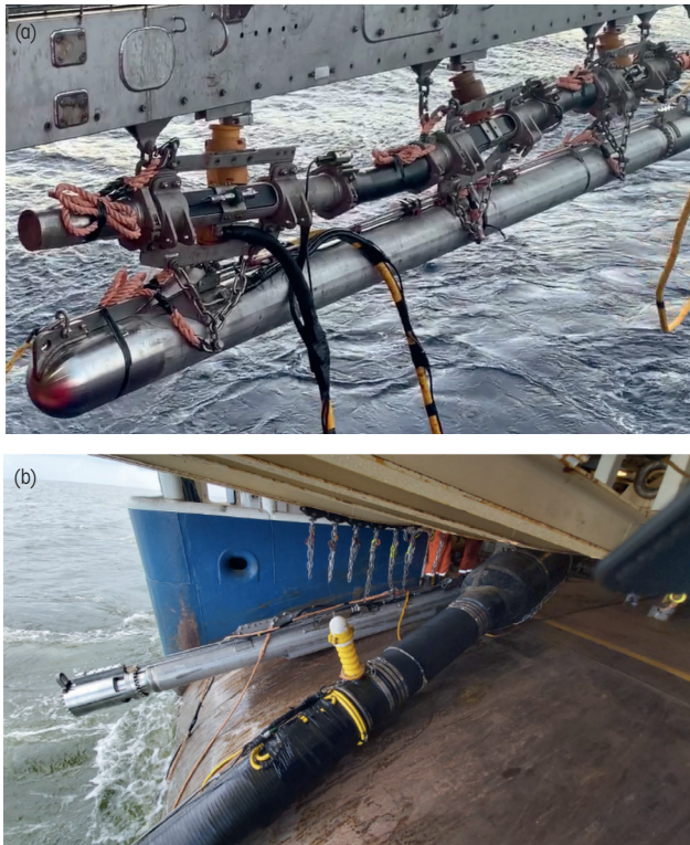
Figure 15 (a) TPS deployed with a boom under a rigid float. (b) TPS deployed on a slip-way together with a flexible float.
