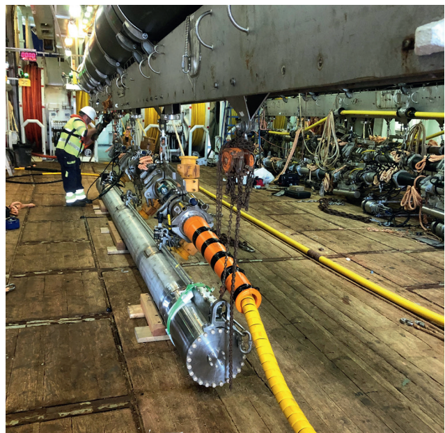
Figure 2 Tuned Pulse Source (TPS) on the back-deck of Sanco Atlantic, Gulf of Mexico, 2020.
