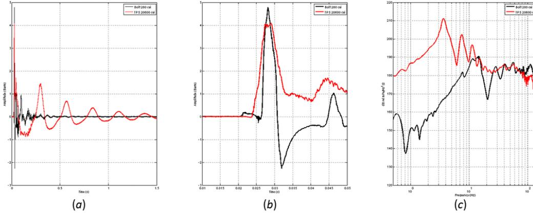
**Figure 2.** Data from the same hydrophone showing TPS versus Bolt. (a) time domain. (b) zoom-in of (a), illustrating the difference in rise time. (c) Spectra of the two signals. Note the 40dB (factor 100!) difference in low frequency signal and a slight reduction in peak amplitude from 4.7 to 4 BarM.
