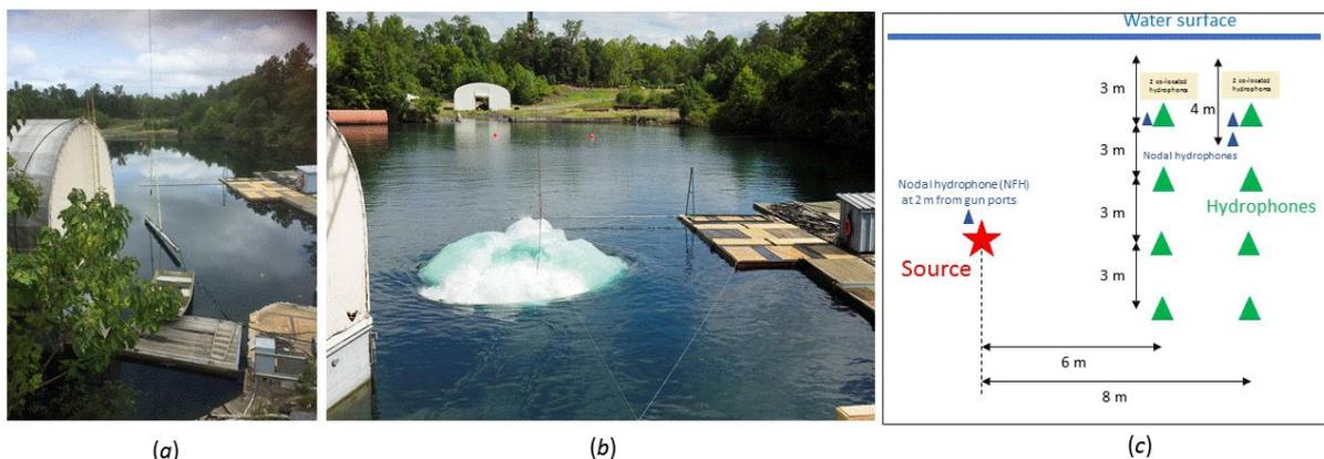
**Figure 1** (a) Deploying the 20,600 cui TPS into the lake, (b) bubble due to source firing at 15 m depth, (c) measurement set-up. A total of 12 different hydrophone locations were present during the test.
