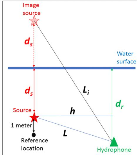
**Figure 3** Nomenclature used in near-to-far-field normalization procedure
