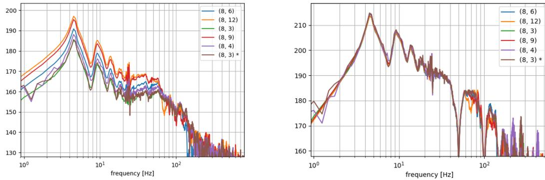
**Figure 4** Spectra of shot at 15 m depth with TPS pressure of 600 psi and volume of 20600 cui. Left: near-field spectrum measured by hydrophones. Right: extrapolation of the measured spectrum to the far field. Numbers in brackets indicate positions of hydrophones as “(horizontal distance to the source, depth)”. The star symbol “\*” refers to the hydrophone at 3-meter depth (a small triangle in figure 1(c)).
