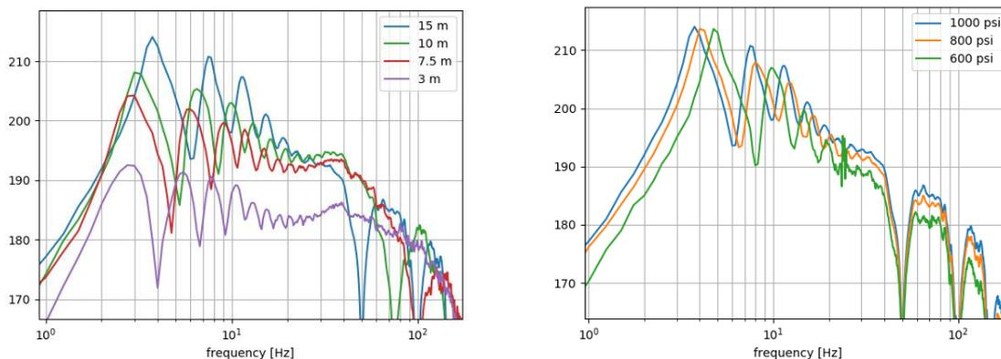
**Figure 5** Dependence of generated sound spectra (dB relative to 1 micro pascal at 1 meter) on source depth (left) and firing pressure (right). The airgun volume is 20600 cui. Left: shots at a pressure of 1000 psi. Right figure shows shots at 15-meter depth. Measured signals have been extrapolated to the far field and averaged over the hydrophone records.
