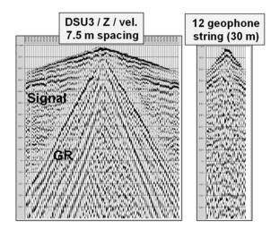
Figure 3: Shot point (GR=ground roll) recorded with single sensor units (DSU) and string of geophones laid out at the same place, but with different spacing. GR is attenuated but it is also aliased on the geophone shot point. (Data courtesy of BNGF).
