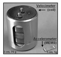
Figure 1: Comparison of a MEMS silicon chip as it is used within digital sensors with the coil/magnet of a geophone.
