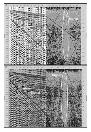
Figure 4: Shot point (GR=ground roll, BS= back scattering) with 10 m spacing (top) and 3.3 m spacing (bottom). (Data courtesy of CGG)
