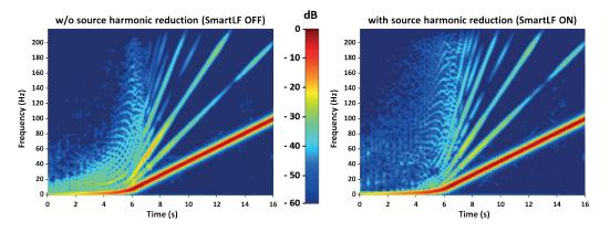
**Figure 2**: Spectrum of the ground force of a shot point, without (left) and with (right) VE464 SmartLF harmonic reduction at the signal emission stage.
