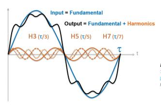
**Figure 1**: an illustration of distorted signal (Output), after the expected "ideal" seismic signal (Input of temporal period  $\tau$ ) has gone through a physical device (source or receiver)
