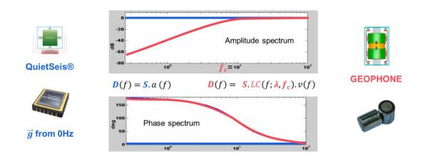
With extremely low manufacturing tolerances and an invariant response to temperature change and aging, QuietSeis MEMS allow for an exact conversion from digital to physical units, which can be acceleration, velocity, or displacement. Additionally, Sercel's manufacturing excellence ensures a certified high-precision orthogonality between the three components.
