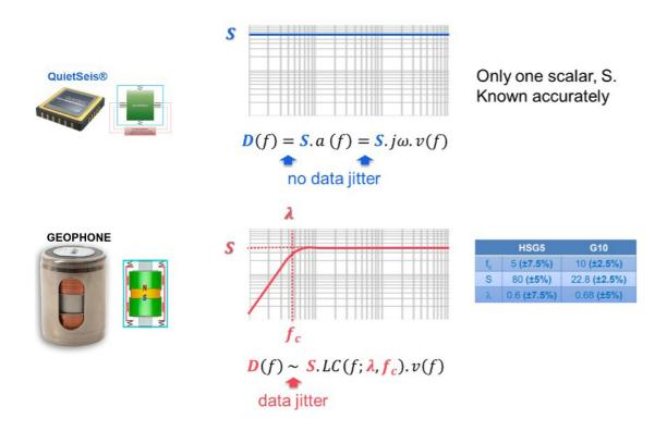
Geophones, on the other hand, involve up to 5 parameters (only 3 are presented in this illustration for the sake of simplicity), all of which vary at the manufacturing stage and during the geophone's lifetime. This creates data jitter, which can easily be observed in the data recorded with geophone-based nodes.
