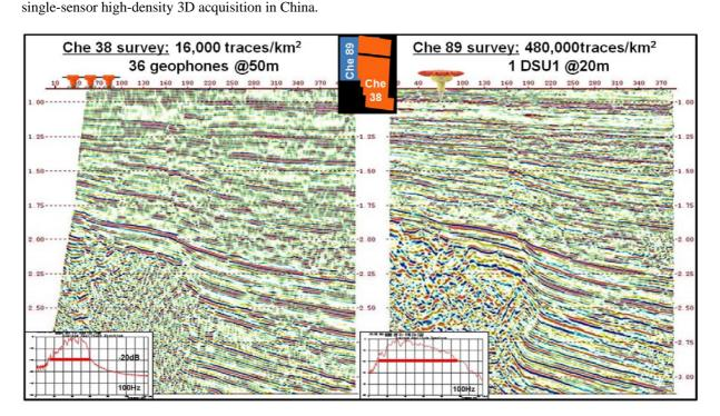
Figure 1: Benefits of single sensor high-density 3D acquisition to improve vertical resolution and seismic imaging.
