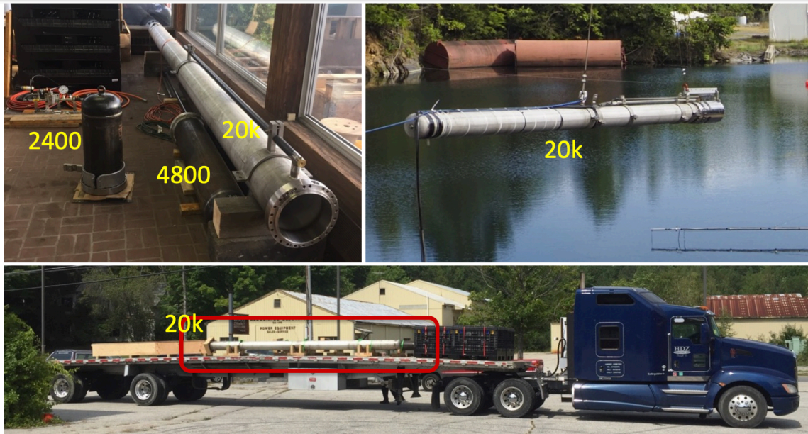
Figure 2. Various volumes of firing chamber that we mounted and tested with the single TPS that we manufactured. Shown here are chambers with 2.4, 4.8, and 20.6 thousand cubic inches.
