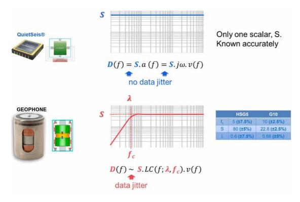
Geophones, on the other hand, involve up to 5 parameters (only 3 are presented in this illustration for the sake of simplicity), all of which vary at the manufacturing stage and during the geophone's lifetime. This creates data jitter, which can easily be observed in the data recorded with geophone-based nodes.
