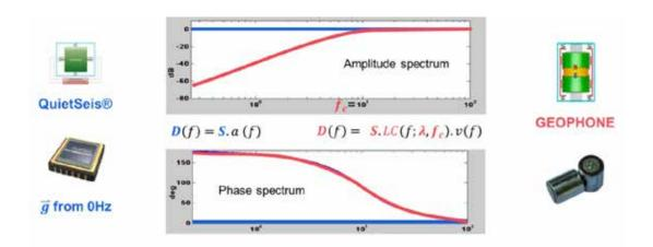
With extremely low manufacturing tolerances and an invariant response to temperature change and aging, QuietSeis MEMS allow for an exact conversion from digital to physical units, which can be acceleration, velocity, or displacement. Additionally, Sercel's manufacturing excellence ensures a certified high-precision orthogonality between the three components.
