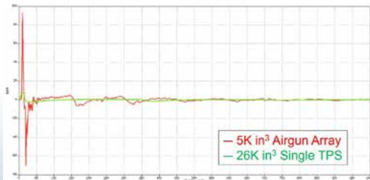
Note that the zero-to-peak sound pressure level of the air-gun array at 92 Bar-Meter is 13 times (22 dB) higher than the TPS at 7 Bar-Meter.
