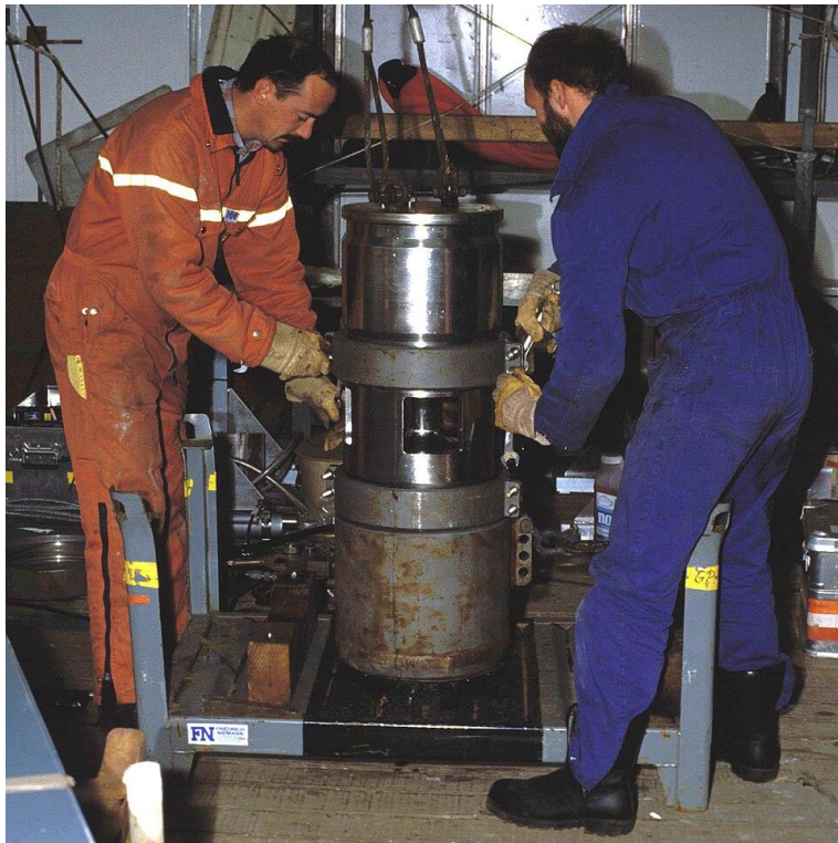
Figure 1 2000 cubic inch Airgun being serviced. These guns were used in a survey that was designed by Ziolkowski et al and was acquired and processed by VeritasDGC in 2001. The head of this Airgun is almost as large as the head of the TPS. The firing chamber, however, is “only” 2000 cui compared to 28000 cui for the TPS. The pressure of this source was 2000 PSI which is double the TPS pressure. So the amount of air discharged per shot of this gun was only factor 7 less than TPS. (Figure from Wikipedia by Grobe, 2006.)
