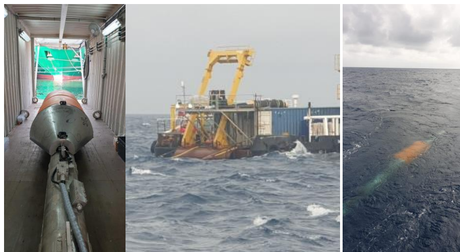
Figure 3 Tuned Pulse Source with an Integrated Float System. Deployed from a fully containerized vessel.
